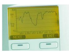
The display can be used to trace measurement trends back for up to a year.
