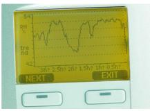
The display can be used to trace measurement trends back for up to a year.
