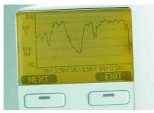
With the help of the display, the user is able to trace measurement trends back for up to a year.
